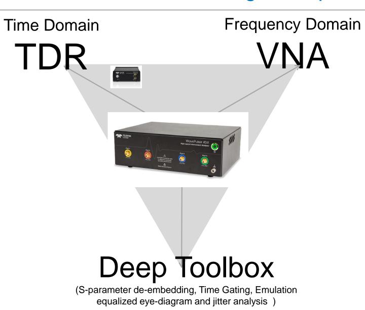
The combination of S-parameters (frequency domain) and Impedance Profile (time domain) in a single acquisition with a deep toolbox for simulation, emulation, de-embedding and time-gating provides:
